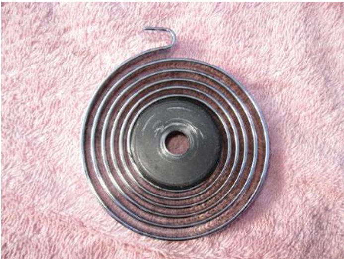
This is now the front / outside / "visible" side of the engine mount with the spring squashed onto the ring. The new threaded rod / engine mount "axle" goes through the hole and a nut fixes fastens the whole thing together.
