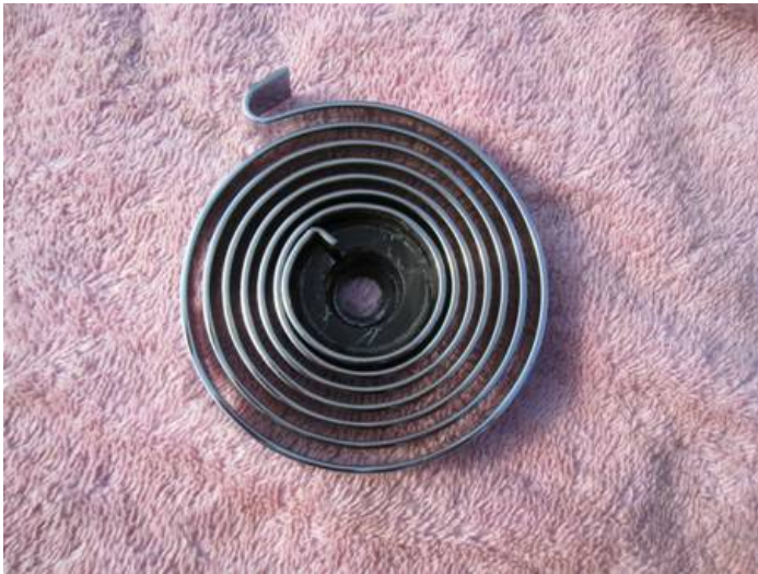
This is the inside with the spring hooked in the newly cut slot / Being the inside it is not visible, the spring is a perfect diameter match - what a coincidence.
