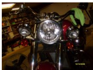
Light bar mounted under headlight bracket with no cover an no freeway bar clearance
