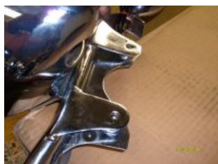
Light bar will not work under headlight bracket
