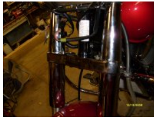
Lower tree cover back in place with shortened side bolts
