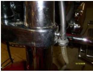
Side signal bar bolts too long
