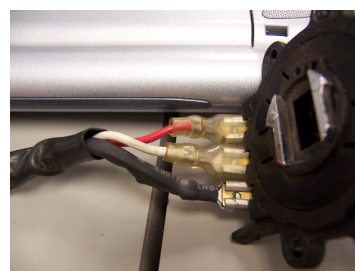
This is a close up of the connections to the Thunder Mfg. switch. You can see the red and the white wires. The heat shrink is hiding the infamous resistor on the third connection.
