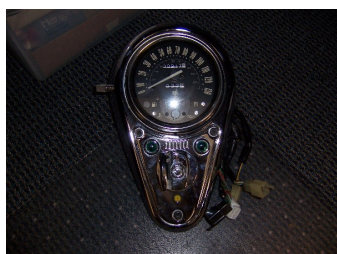
The H-D style switch mounts upside down so the door opens opposite from those on Harleys
