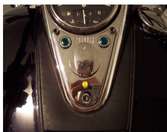
This is the Thunder Mfg. Dash mount ignition switch on my 2000 Kawasaki Nomad FI (4.2 gallon tank and mechanical speedometer cable)
