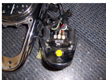
The Thunder Mfg. switch and panel viewed from the back.
