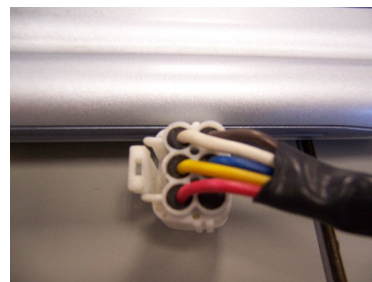
A close up view of the OEM style plug and the five wires. The wire colors appear to be red, yellow, white, brown and blue with the sixth slot open or free.
