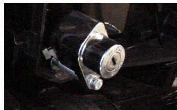
Cover Off, Close Up Of Standoff & Longer Bolt
