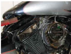
Remove the instrument cluster surround and the front and rear attaching bolts for the tank then raise the rear of the tank. This will give you access to the throttle bellcrank.
