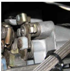
This photo is with the fast idle knob pulled out. Notice how the nylon spacer is pushing down on the lever holding the throttle open just slightly. You can tune the cold idle rpm by sanding or filing more or less from the bottom of the spacer.
