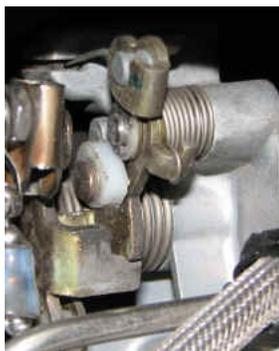
Before installing using a file, grind a little bit off one side (this will become the top) to clear a washer on the throttle mechanism (see photo below left)
