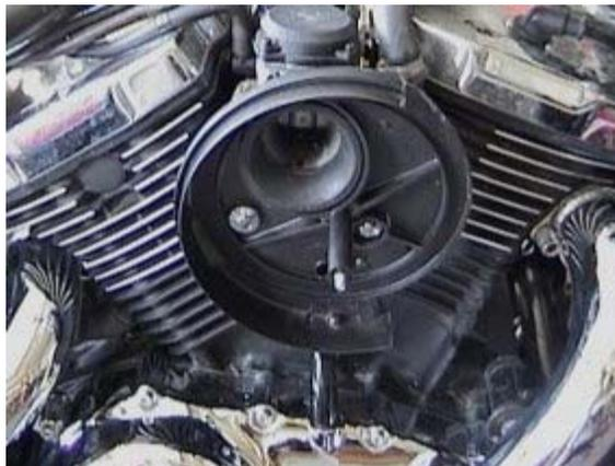
**f.** Reinstall completed backplate on carb.
