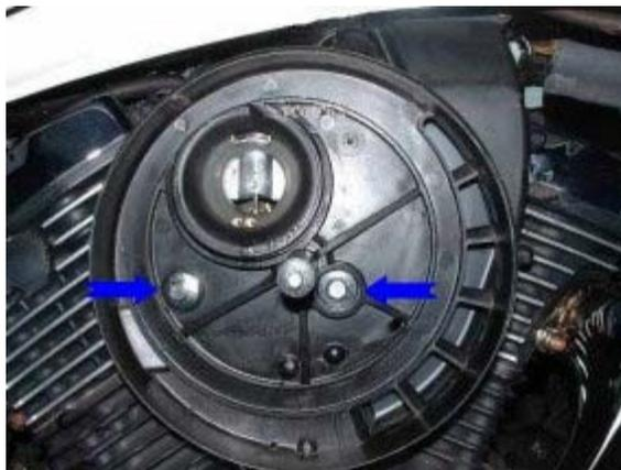
e. Remove the 2 10mm bolts holding the backing plate to the securing bracket in front of the carburetor. Set these bolts aside someplace safe; *they will be reused.* Carefully ease the backing plate off the carburetor.
