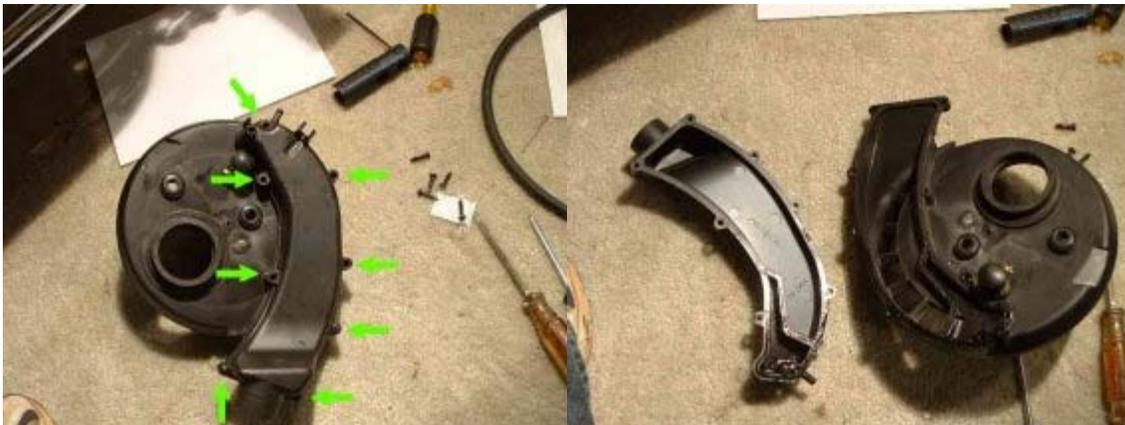
a. Remove the 8 Phillips head screws holding the back of the snorkel to the backing plate. Dispose of this snorkel half and the screws; *once the backplate has been modified, they cannot be reused.*
