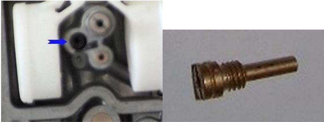
e. Remove the Pilot jet. Be careful not to hit the floats. Put the OEM Pilot jet (**48**) in a spare parts bin; *it will **not** be reused*, but may be necessary to reinstall should the bike ever need to be returned to factory original settings. Install the **50** (used with aftermarket needle) or **52** (used with OEM needle) Pilot jet. Tighten down only until seated firmly.
