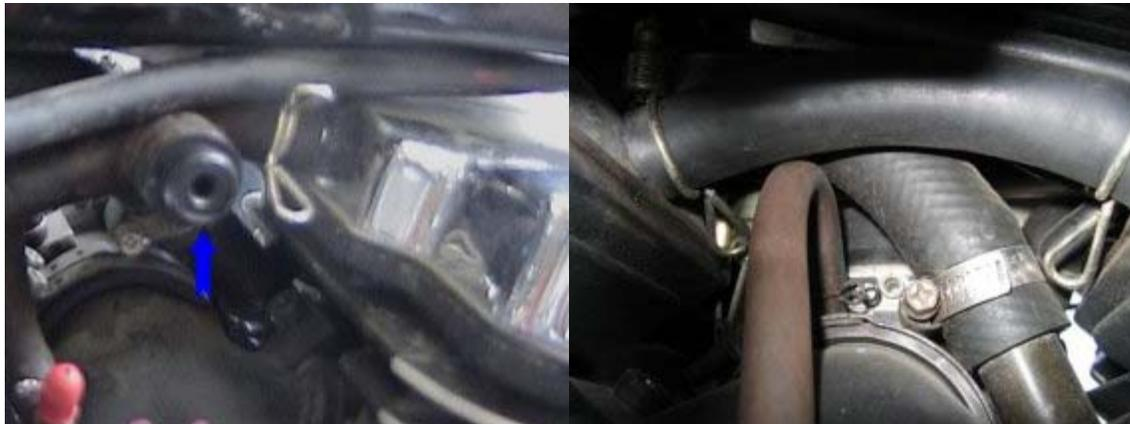
**b.** The reed valve line is a T-shaped hose that connects the two reed valves (in the cylinder heads) and the switch valve. Either plug the hole in the line to the switch valve (a large marble or internal line plug works well), remove the line and install vacuum caps over the nipples (better solution), or remove the line and replace it with a single length of high-temperature, high-pressure radiator line (best solution). This blocks the operation of the reed valves.
