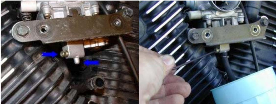
**a.** Drain fuel from carburetor float bowl by opening the 3mm Allen head bolt (carburetor drain plug) next to the small nipple on the bottom of the carburetor (carburetor drain). Catch this fuel in a non-flammable container (do *not* use a Styrofoam cup; gasoline will dissolve Styrofoam). Dispose of this fuel safely and immediately. Tighten drain plug.
