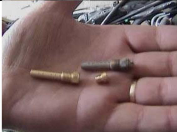
**CAUTION!** Do not allow the bottom of the carb to face down while the Main jet is removed! If the bottom is down, there is a chance that the needle seat above the Main jet will fall out; this is a small part that will be difficult to locate and reinstall if it does. Should the needle seat fall out, *very carefully* reinstall it with the thick side facing the Main jet.
