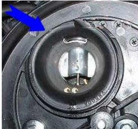
Note the position of the black rubber boot between the backing plate and the carb, and that the boot *is* rubber and *must not* be damaged. Set the backing plate aside someplace safe; *it will be reused*.
