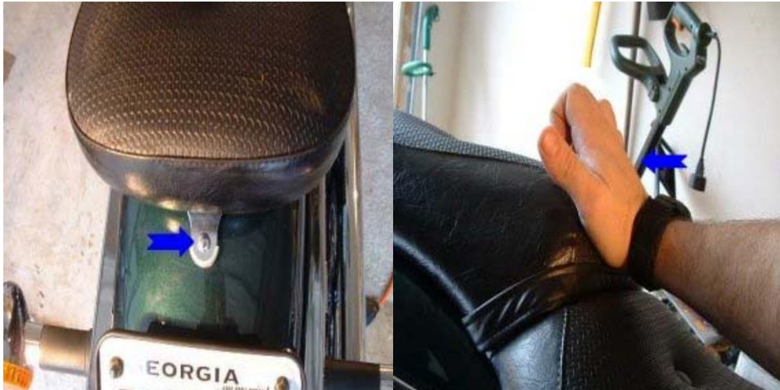
Remove the 8mm bolt at the rear that holds the back of the seat onto the fender. Strike the back of the rider's section of the seat (the "step" where it comes up to become the passenger seat) solidly toward the rear of the bike to release the clips holding the seat onto the U-bracket on the rear fender. Lift the rear of the seat and pull backwards; the front tab will come out from underneath the rear bolt of the fuel tank. Set the seat aside someplace safe.
