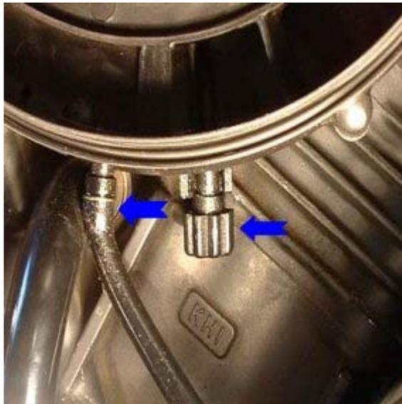
d. The idle RPM adjust is a black plastic knob hanging to the lower right of the backing plate; it is secured on a small clip to the rear of the backing plate. Pull the line clear of the clip and allow it to hang. Disconnect the small line just to the left of the RPM adjust. This is the line that goes to the “milk bottle” at the front of the frame. Remove this line and the bottle. Put both line and bottle in spare parts bin; *they will not be reused.*
