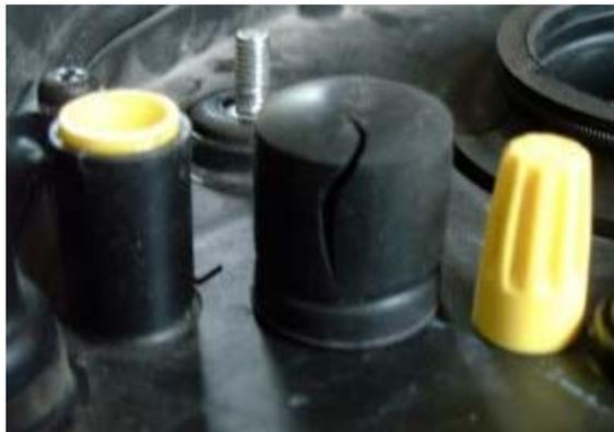
Alternate (updated) method to plug the large nipple; spread some RTV gasket sealant (**Permatex Blue**) over a yellow 12-18 AWG wire connector and insert it small-end down into the nipple. In picture; on left, installed plug. Center, original vacuum cap which had deteriorated and cracked, necessitating replacement. Right, exemplar wire connector.
