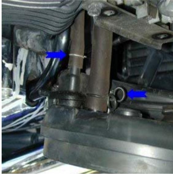
c. Disconnect and label the crankcase vent line (small hose) and the air switch valve line (large hose) from the rear of the backing plate.
