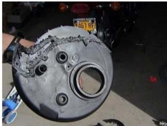
c. With the snorkel ridges cut down, cut the *entire* section containing the deflector vanes away. Smooth down the cut surfaces.
