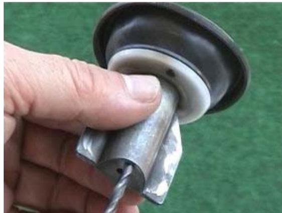
Note the position of the drill bit; *do not drill the center hole!* Using a  $1/8''$  drill bit and drill motor, *carefully* drill through this hole, thus enlarging it. It is *essential* that the bit follow the vertical alignment of the original hole.
