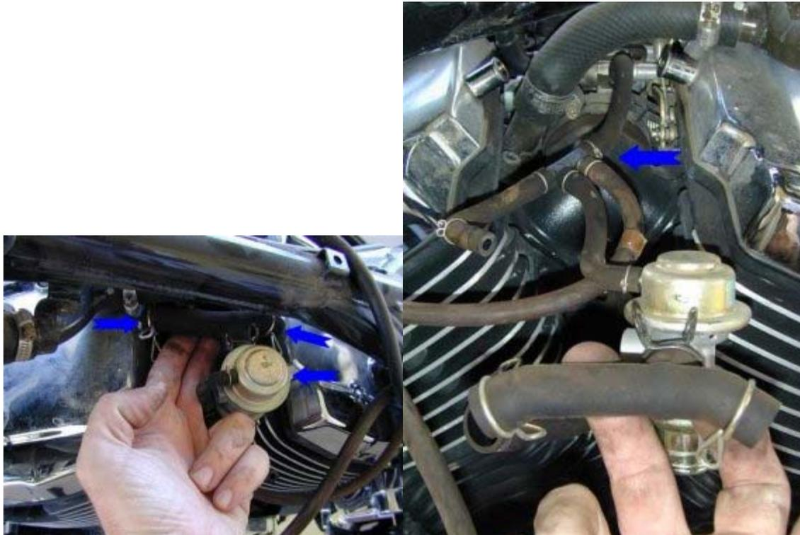
**a.** Release the clamp holding the reed valve line to the switch valve and the clamp holding the vacuum line from the carburetor to the switch valve. Pull the switch valve free of both lines; the third line going to, and previously removed from the airbox backing plate will come free with the switch valve. Put the switch valve, line, and clamps in a spare parts bin; *they will not be reused*, but may be needed should the bike ever need to be returned to factory original configuration.
