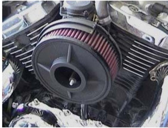
g. Install new **K&N** air filter onto backplate.
