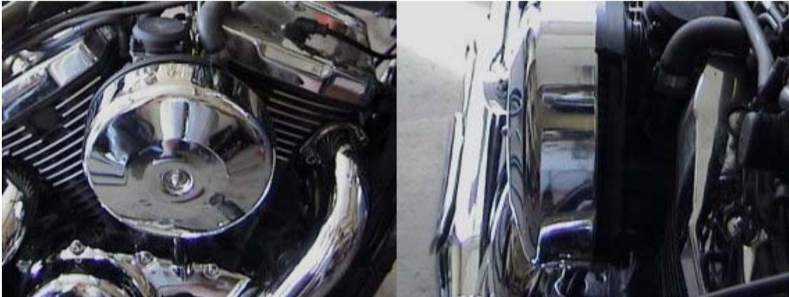
h. Install chrome cover. Note the large opening now available for air to flow into the air cleaner. There will now be plenty of air available for the engine.
