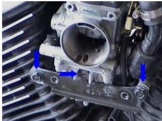
**b.** Remove the 2 10mm bolts holding the airbox mounting bracket/carburetor stop in place. **Caution:** These bolts are harder than the
