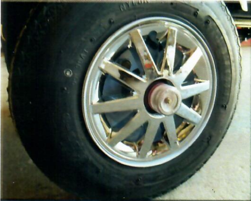
STANDARD WHEEL W/HUBCAP & BUDDY BEARING 4.80 x 8
