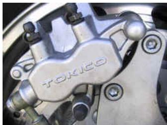
12. If you're doing the rear it is done exactly the same as the fronts except rather than hex bolts you have 8 mm Allen head bolts holding the caliper in place. Loosen and remove these bolts, lift the caliper off the disk and change pads exactly the same as above. When finished tighten the Allen bolts to 25 foot lbs.
