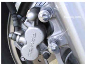
1. Loosen the caliper bolts (both sides of wheel for Nomad) With the bolts removed lift the caliper off the disk taking care not to support the full weight of the caliper by the hose. It might help if you un-clip the hose where it's attached to the fork at the reflector.
