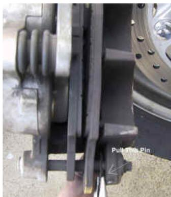
2. Rotate the caliper so you're looking at the pads. Note a pin running across the bottom that's held in place by a pin. Remove the pin (see arrow in photo) and put it someplace safe.
