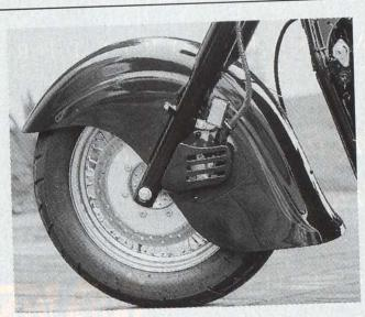
Reminiscent of a luxury car from the 1930s, that full, sweeping fender sets the bike apart from any other current model. It shrouds the caliper for the more powerful front brake, which is one of the functional advances of this new/old motorcycle.
