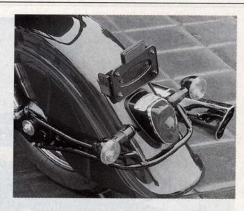
To give the fender the low profile available on a motorcycle without rear suspension, it was mounted to the swingarm and wrapped snugly around the wheel. Many of the pieces on this prototype, including the seat rail and shocks, will change.
